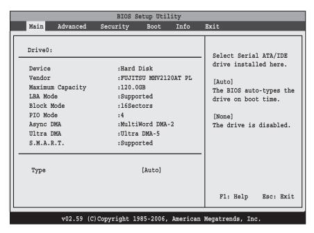
Figure 2. Drive0 Master Submenu
